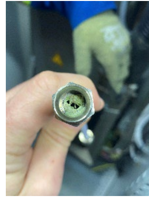
Figure 4 Solid Deposits Inside Hot Sample Pump
