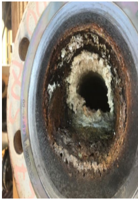
Figure 2 Heavily Corroded Stack Mounting Flange
