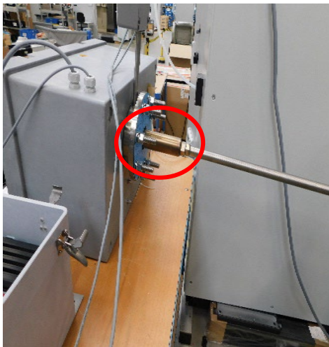
Figure 6 – Sample Probe Heated Transition Piece
